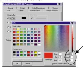
Match the RGB values after setting the cut lines' [Weight] to Opt in the Illustrator 7.01. If not, it can not be cut.
